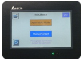
Touch Screen Automatically Adjusts Side Seal, Inverting Head and Infeed Conveyor
