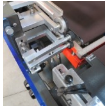
Film Miser - helps track film allowing for smaller width film rolls to save money
