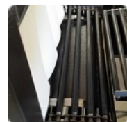
High Density Rollers - Close Roller Spacing 1/2" Gap
