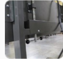
Crank Handle to Move Tunnel Chamber Up or Down
