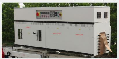
• Heat 3 & Heat 4 is for left and right infrared heating bar pointed to the jar's neck. (With yellow label)
