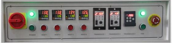
Heat 1 & Heat 2 is for dual zones heating of infeed part. (With yellow label on machine)
