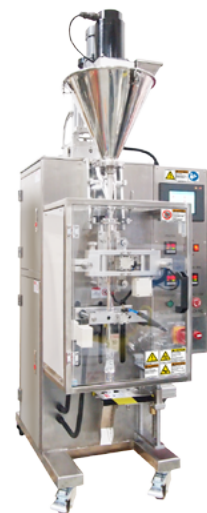
(Above) The R95-AG Vertical Stick-pack FFS with Auger Filler
