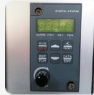
Variable Air Velocity Control
