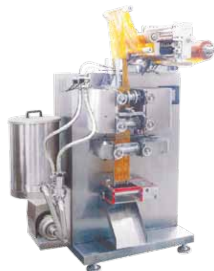
(Above) The 6 Series Sachet FFS, single lane model 65-LC.
