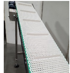
1" tall cleats spaced 10" apart help transport products up the conveyor
