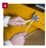
**1** Eject the finished bale after compacting waste. **2** Remove and store finished bale until pickup. **3** Using the safe two-hand ejection system, the finished bale is ejected automatically. **4** Knife mounted on front of baler allows safe cutting of straps.
