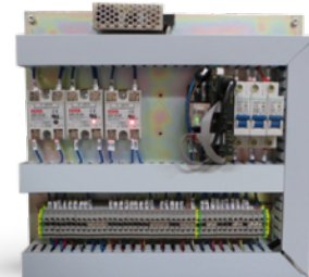
Solid state relays for reliable operation. Panasonic PLC
