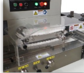
Top brush helps evacuate air from bag and controls spacing. Includes infeed and discharge safety covers.
