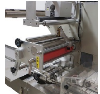
Optional date coder, thermal transfer or inkjet printer for printing expiration date, sell-by date or lot number.
