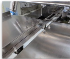
Flighted infeed with product carriers makes transporting sticky products much easier.
