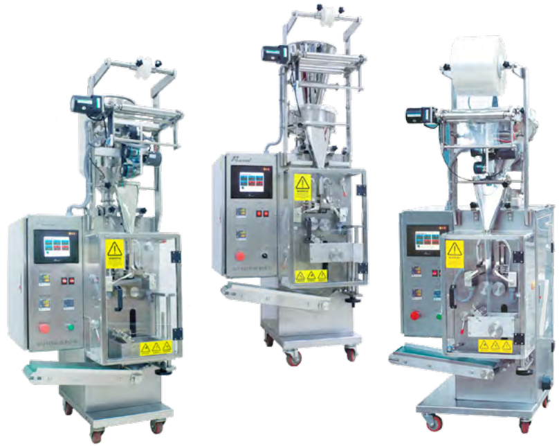
(Top) The stainless steel construction 5 Series Sachet FFS equipped with volumetric piston filler (left), volumetric turntable filler (middle), auger screw filler (right).
