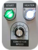
Variable Speed Control 0 - 75 FPM
