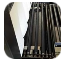
High Density Rollers - Close Roller Spacing 1/2" Gap
