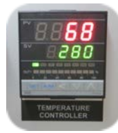
Digital Temperature Control 0-400° F
