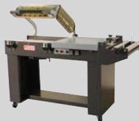
PP-3040HK Hot Knife Seal System Used with Polyethylene Films.
