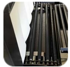
High Density Rollers - Close Roller Spacing 1/2" Gap
