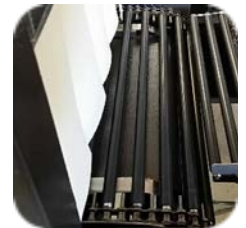
High Density Rollers - Close Roller Spacing 1/2" Gap
